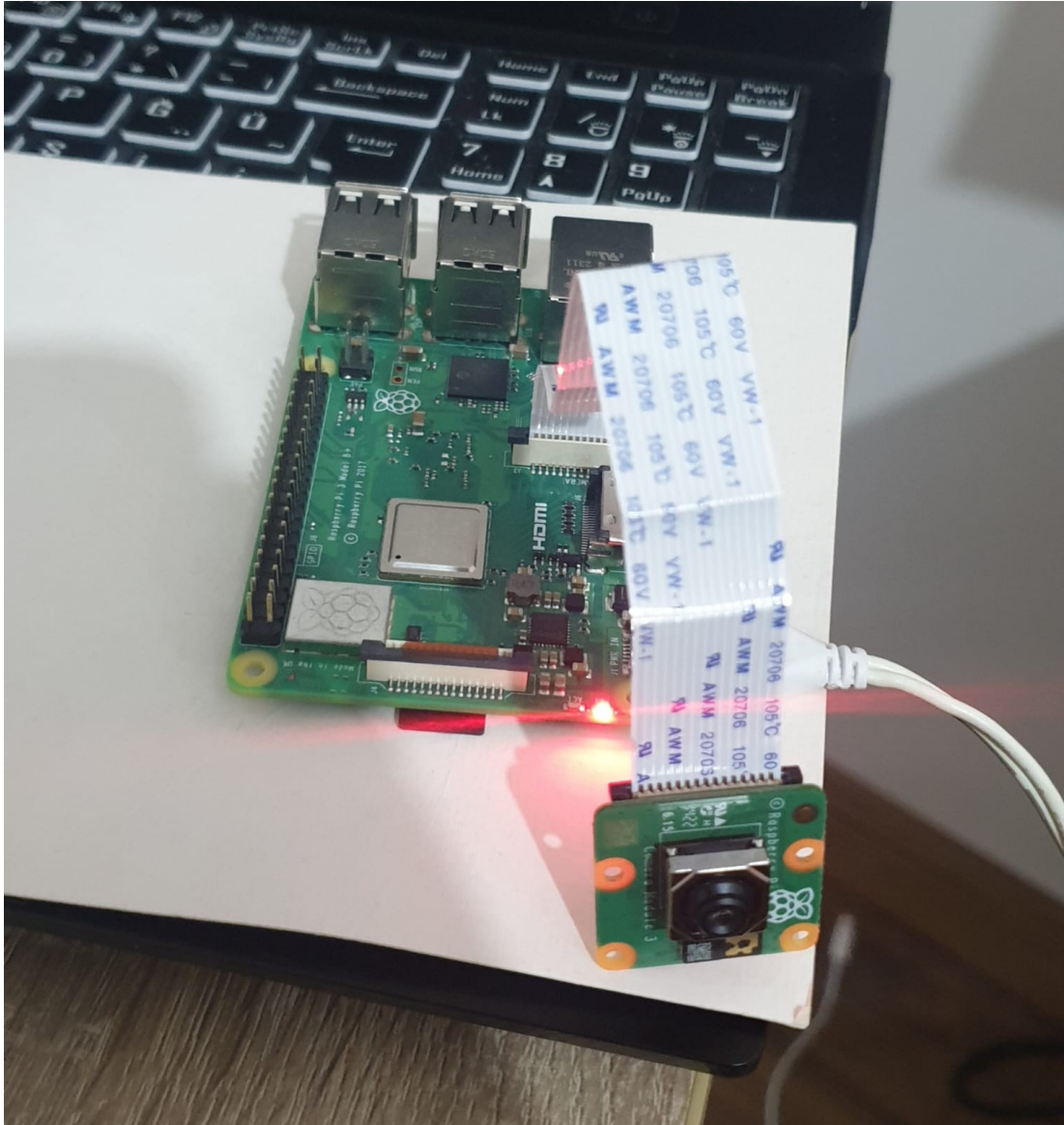
Figure 3.2: Photo Of the Raspberry Pi with Camera Module 3.
